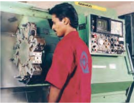
20 HP CNC chucker for heavy stock removal
