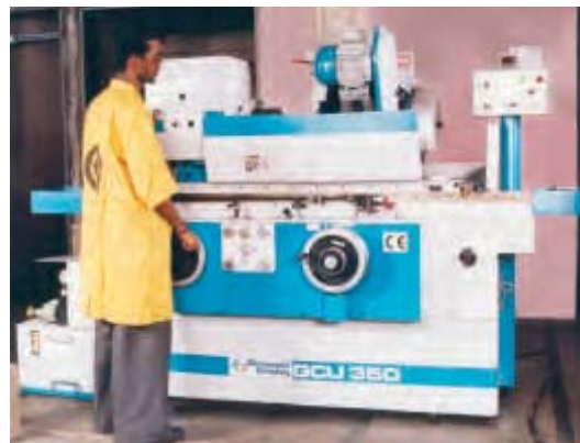
Universal Hydraulic Cylindrical Grinder with Diamond wheels to machine hard seal components
