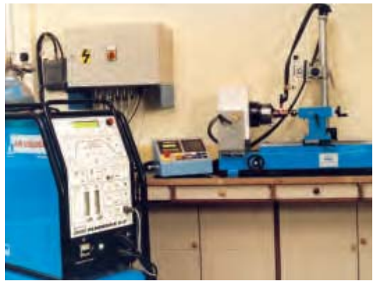
State- of- the- art facility for Metal Bellow Seals welding
