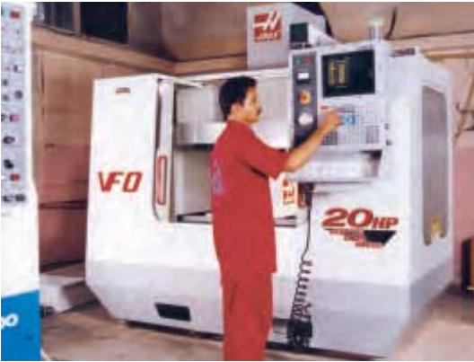
20 HP, 4 Axis Vertical Machining centre for complex milling / drilling operations
