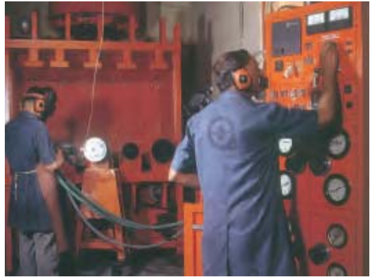
Advanced High-energy Plasma -Thermal spray system for production of wear - resistant coatings
