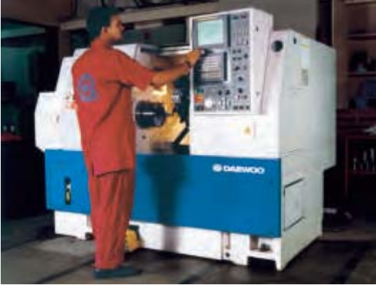
11-KW CNC Lathe for rapid Production of seal components
